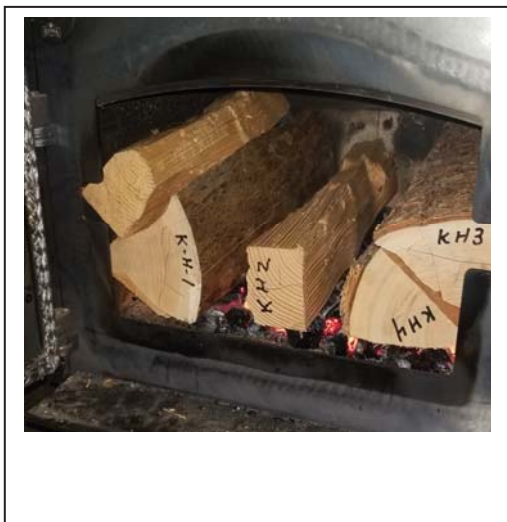
Run 1 – Test Fuel Load In Stove
