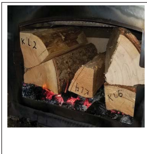
Run 2 – Test Fuel Loaded into Stove
