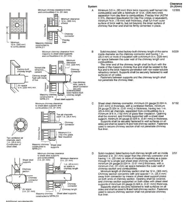
Insulation material used as part of wall pass-through system shall be of noncombustible material and shall have a thermal conductivity of 1.0 Btu-in./hr-tft<sup>2</sup>-'F (4.88 kg-cal/hr-m<sup>2</sup>-'C) or less.
