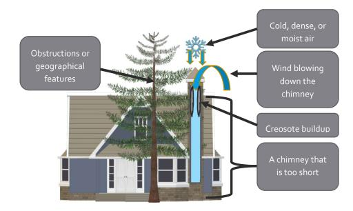
**Too much draft** may cause excessive temperatures inside the firebox and may damage the internal components of the stove. An uncontrollable burn or excessive temperature indicates excessive draft. **Factors that increase draft are:**
