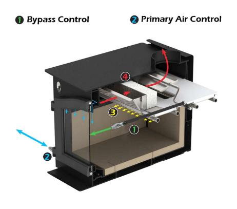
Secondary Burn System @Catalytic & Catalytic Thermometer
