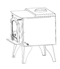
**Step 5:** After 15 minutes, or once the catalytic thermometer enters the active range, close the bypass control engaging the combustor (Simply lift the bypass control and you will feel it return to the closed position). Leave the air control open for 20-30 minutes so that the fire becomes well established. If you shut the stove down too soon, it may go out or the combustor may stop working.
