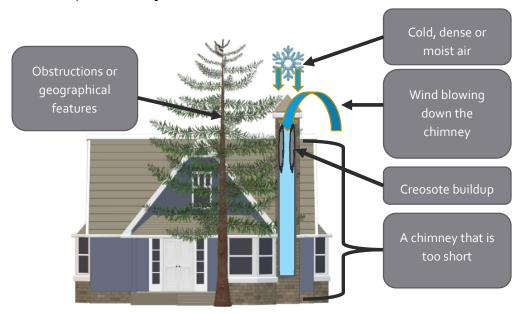
Too much draft may cause excessive temperatures in the appliance and may damage the internal components of the stove. An uncontrollable burn or excessive temperature indicates excessive draft. Factors that increase draft are:
