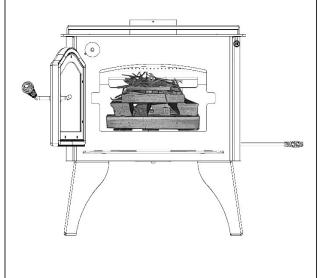
**Step 4:** Light the Fire, you can optionally leave the door slightly cracked open to aid in the start-up of your stove. Close the door once the fire is well lit. **Do not leave the stove unattended with the door open.**
