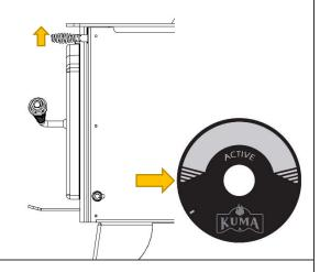
**Step 6:** After 20-30 minutes, begin to regulate the heat output and burn rate by sliding in the air control. Use the table below to adjust your rate of burn:
