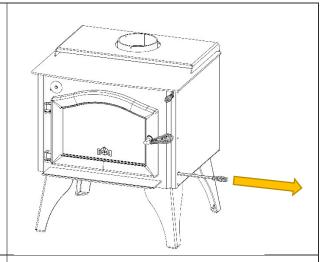
**Step 2:** Pull the bypass control open: a short pull toward yourself (about ¾") and down will open the bypass allowing the chimney to heat quickly. This also prevents smoke from coming into the room when the door is open.
