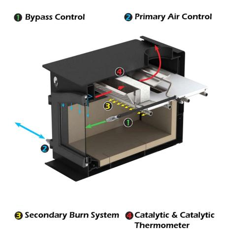
1. **Bypass Control** – Located on the upper right side of the stove, the bypass control allows smoke and heat to temporarily bypass the hybrid burn system. This helps to quickly heat the chimney and prevent smoke from coming into the room when the door is open.
