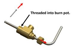
**STEP 1**: Remove the cotter key from the end of the decoker. Use pliers to straighten the cotter key then pull out. Unscrew the gasket nut.
