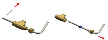
**STEP 2**: Disassemble the decoker assembly. Remove the cotter key with pliers and unthread the gasket nut with a 9/16 or 15mm wrench. Pull the complete rod assembly out of the decoker body. You must save the gasket nut and the small brass ring. The old decoking rod, gasket, and cotter key will not be reused.
