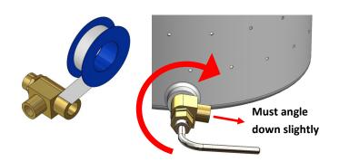
**STEP 6**: Apply several wraps of thread tape in the direction shown. Thread the decoker assembly into the burner and tighten with the adjustable wrench. The fuel line connection must angle down slightly as shown.
