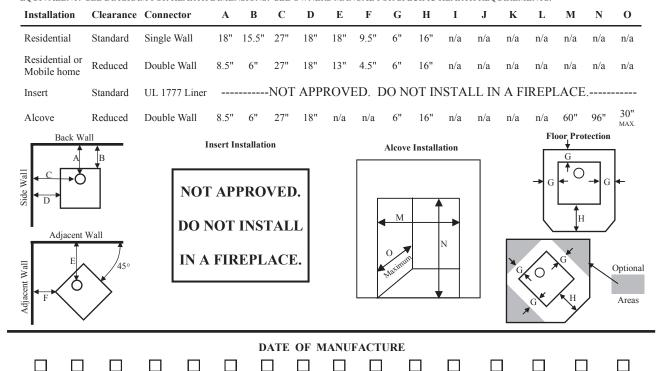
U.S. ENVIRONMENTAL PROTECTION AGENCY: Certified to comply with 2015 particulate emission standards. Not approved for sale after May 15, 2020. 3.5 Grams per hour. Tested to EPA method 5G-1 and EPA method 28. Complies with May 15, 2015 crib wood standards.
